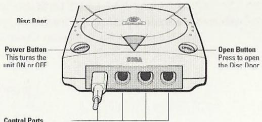
Use these ports to connect the Sega Dreamcast Controller or other peripheral equipment. From left to right are Control Port A, Control Port B, Control Port C, and Control Port D. Use each port to connect controllers for players 1 to 4 respectively. NOTE: Control Port can also be referred to as Port
